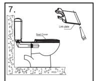
Measure and mark the area to be cut from the link plate by loosely installing the toilet seat into the pan. Remove both items and make the cut with a fine tooth hand saw/hacksaw. Note - Use the cut lines on the back of the link plate to ensure you achieve a straight cut. Reinstall the link plate.
