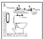
Hang the bracket on the wall. Note - Take caution when selecting the area to be drilled as water pipes or other hazardous objects may be present in wall. Install the cistern
