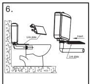
Install the link plate on the cistern.
