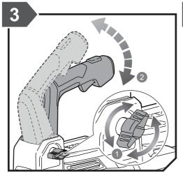
Turn the handle adjustment knob clockwise or counterclockwise. Lift the handle.
