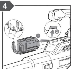
Install the battery pack. Make sure that the latch on the battery pack clicks into place. Press the trigger to turn on the product.
