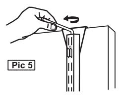
Tighten the screw in the Top Bracket using the Allen Key supplied. (Pic 5)
