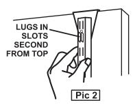
Attach the Wallstrip by inserting the lugs of the Top Bracket into the slots which are second from the top of the Wallstrip. (Pic 2)
