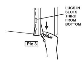
Attach the Bottom Bracket to the Wallstrip by inserting the lugs into the slots which are third from the bottom of the Wallstrip. Pull the Bracket down and secure under the door. (Pic 3)
