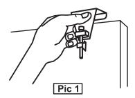
Hook the Top Bracket (with the screw mechanism) over the top of the door. (Pic 1)
