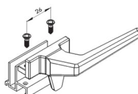
\*Note: Sub fix handles can replace most vertical fix handles by re-aligning fixing holes.
