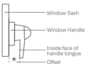
Should the offset vary from standard size, the difference can be made up with self adhesive wedges as seen here:
