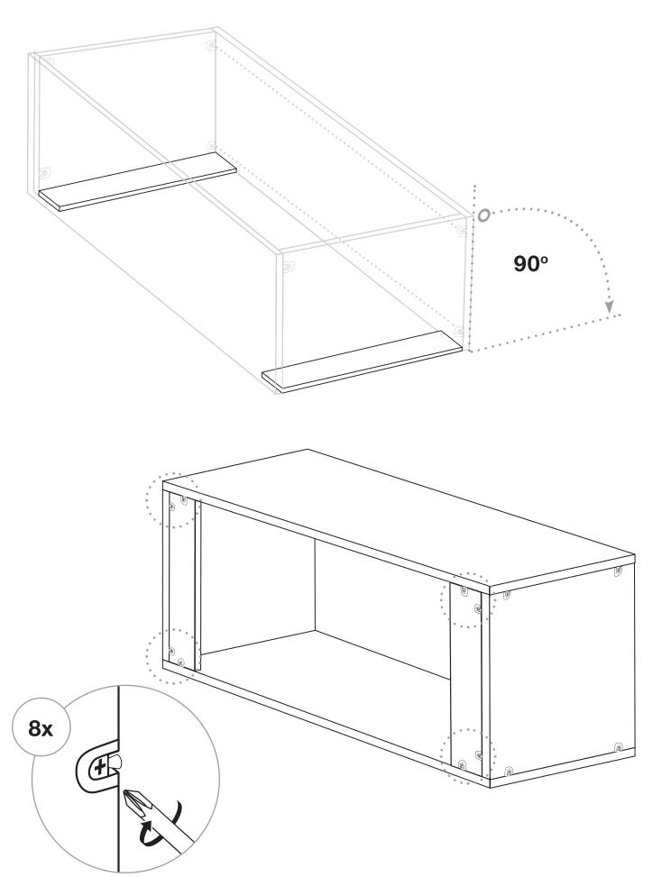
Rotate the cabinet 90° on to it's front - so that the back of the cabinet is facing up.
