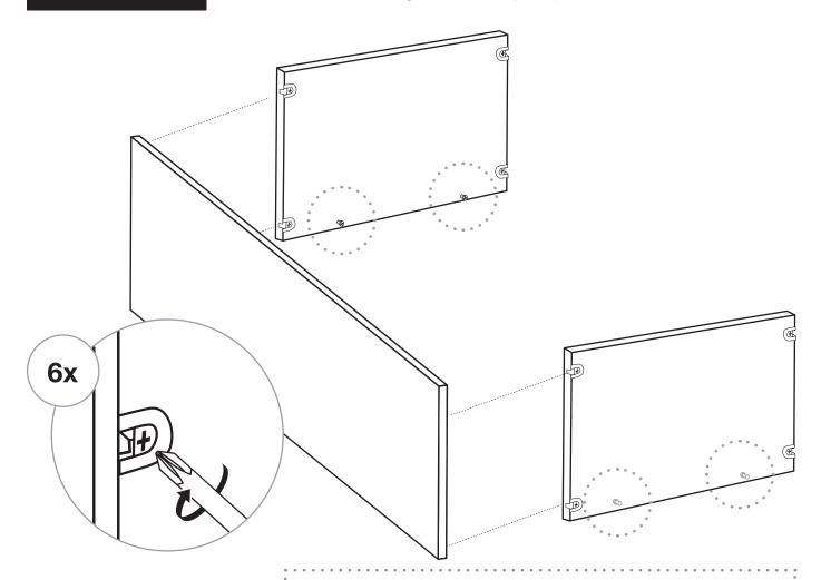
Note – The Cam Lock Screws on the Top and Base should point to the inside of the cabinet. Rotate the panels so that the Cam Lock Screws are on the floor.
