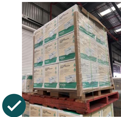
Figure 17 – Example of correct use of corner posts
