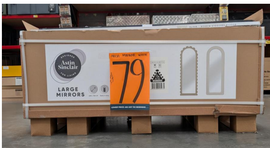
Figure 12. Example of 60 kg+ item built in cardboard skid with sufficient clearance for manual handling equipment.
