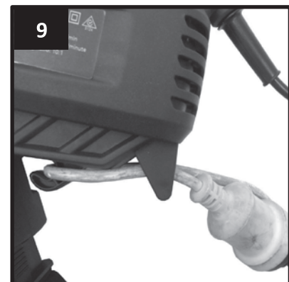
9 Make a loop with the extension cord and push it through the square hole under the motor housing and over cord retainer. Connect the extension cord socket to the blower vac's cord plug.
