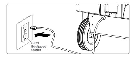
**NOTE:** A live power outlet can be verified when the Cooling Unit is **plugged in and powered off** by pressing the **oscillation** or **water** buttons. The LED lights will dimly illuminate when either of these buttons are depressed.
