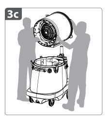
**3c.** Once again, lift the **fan head** and **align it with** the **fan head support pole**. Turn the **fan head** until you feel it engage.
