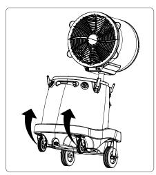
**NEVER install or rotate fan head so that if faces the away from the tank.** Doing so may allow the Cooling Unit to become unstable and create a tipping hazard.
