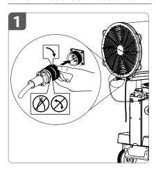
Insert **fan head power connector** into fan head. Ensure female end of power connector is aligned to male connector and *twist* together.
