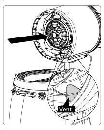
If you see a collection of dust or debris in the head of the Cooling Unit, clean the Cooling Unit with a hose.
