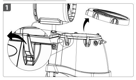
Unlock lid latches (4) and remove lid. Ensure both rear wheels are locked.
