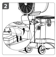
Remove water inlet hose from the front hole in the tank.
