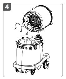
Once installed, the **atomizer** (metal disk) will be facing the **tank**, air will be blown *over* the **tank** when the Cooling Unit is turned on.
