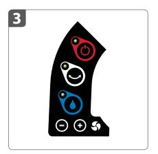
The **LED lights** on the **control panel** will flash in approximately 10 seconds after the Cooling Unit has been plugged in.
