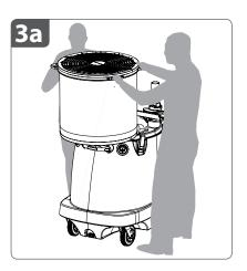
**3a.** Lift the **fan head** straight up and out of the **tank**. Carefully rest it on the **edge of the tank** opposite of the **fan head support pole**, as shown.
