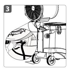
Depress **bulkhead fitting** with one hand while pulling **water inlet hose** with the other hand to remove.
