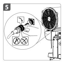
Reconnect the fan head power connector to the bulkhead fitting.
