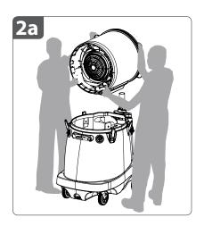
**2a.** Lift the **fan head** straight up and off the **head support pole.**
