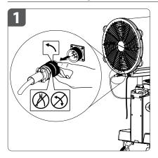
Disconnect the **fan head power connector** from the **bulkhead fitting**.
