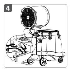
Insert atomizer drain hose into the front hole on top of the tank, from where the water inlet hose was originally removed.
