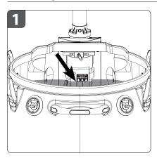
Do not fill the tank above the **max fill level**, as shown. If tank is filled past this level, water may leak out of the tank and cause a hazard around the Cooling Unit.
