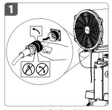
Disconnect the **fan head power connector** from the **bulkhead fitting** if not already disconnected.
