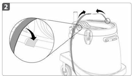
Secure the Cooling Unit by wrapping a band around it, following the grooves on the tank with the strap.
