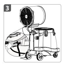
Insert water inlet hose into bulkhead fitting. Ensure that connection is sealed.
