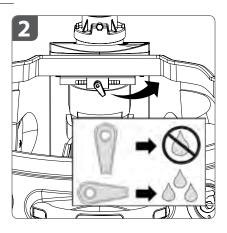
The **water valve** can be adjusted for optimal performance according to climate. To adjust, please follow the steps on the next page.
