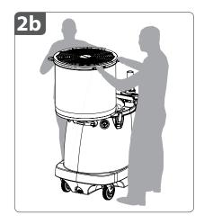
**2b.** Carefully rest **fan head** on the **edge of the tank** opposite of the **head support pole**, as shown.
