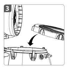
Once tank has been filled to the desired level, place **lid** on tank and close all **lid latches** (4).
