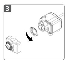
Remove locking ring by turning counter clockwise.
