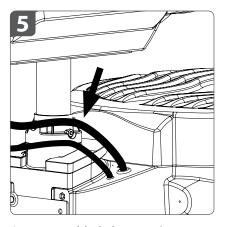
Once assembled, the **atomizer drain hose** should be flexible, but not so loose that water gets backed up in the hose.
