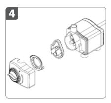
Pull impeller cover to remove it.
