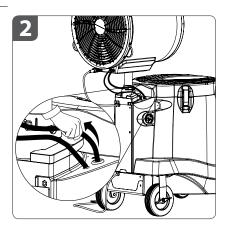
Take **atomizer drain hose** out of the front hole on top of the **tank**.
