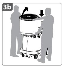
**3b.** Adjust your grip so that each person has one hand on a **strap** and one hand on the **bottom** of the **fan head.**
