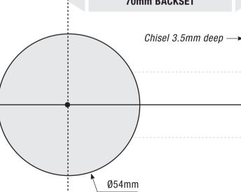
Mark and drill holes from both sides of the door.
