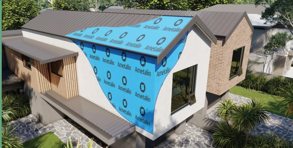
SilverSark® Extra Heavy Duty radiant barrier is designed for multi-purpose use as both roof sarking and a wall wrap. It is suitable for use in all roof and wall types. The reflective foil side provides extra R-value when installed facing an air cavity, and the multi-layer structure provides superior strength, flexibility and durability. Classified as a Water Barrier and Class 2 Vapour Barrier, SilverSark® acts as a barrier to air, radiant heat, moisture ingress and dust penetration.
