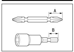
Use only driver bit/socket bit that has inserting portion shown in the figure. Do not use any other driver bit/socket bit.
