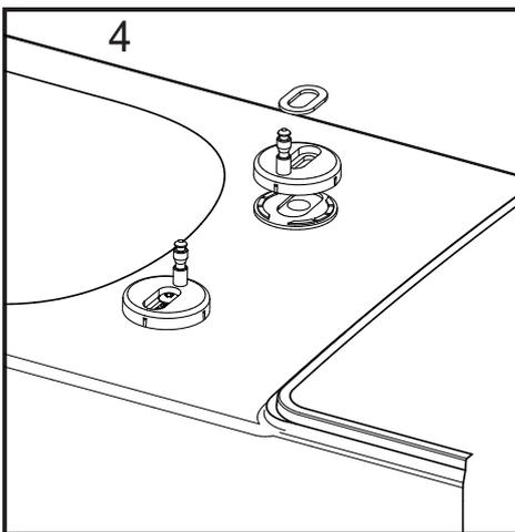
Ensure the rubber pads are fitted to the underside of the hinge mounting posts, insert the elongated washer and loosely fasten to the pan.
