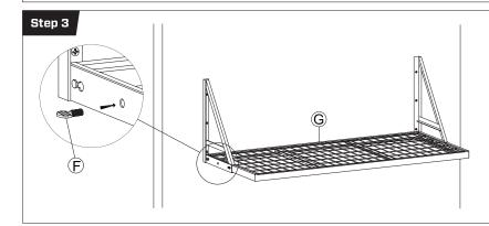
Lay wire shelf (G) on completed frame (A, B, C). Use wing screw (F) to lock the wire shelf in place.
