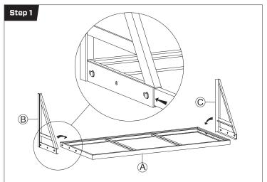
Slide bracket 'B' onto frame 'A'. Use a rubber mallet to tap bracket into place if required. Repeat with bracket 'C'.
