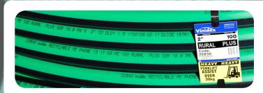
Rural PLUS® polyethylene pipe from Vinidex is specially designed for rural applications. Rural PLUS® Polyethylene pipe is available in diameters ranging from 3/4" (19mm) to 2" (50mm) and can be used at pressures up to 900kPa (PN9) at 20°C.
