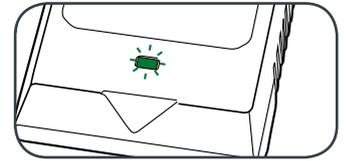
3 With the battery sitting on a flat surface, align the raised ribs on the battery with the recess in the charger and slide onto the battery ensuring a firm connection.
