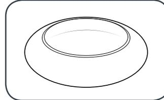
The application bonnet (towelling material) should be used to apply polishing compound to the surface.
