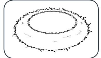
The polishing bonnet (fleece material) is used once the polishing compound is applied and will remove the compound leaving a polished surface.
