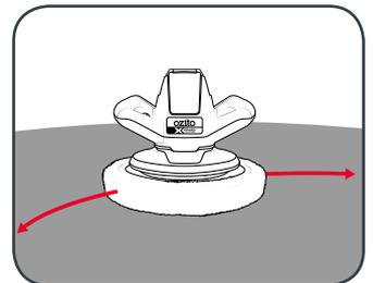
**Note:** Do not apply excessive force to the polisher. Allow the polisher to do the work.
