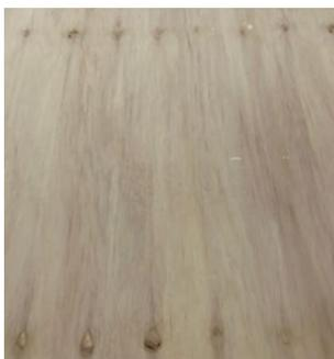
CD - C quality front/D rear face. Sound knots less than 50mm and open defects on the face are filled and sanded. Applications could include substrates for membrane systems, formwork, flooring, roofing and bracing.
