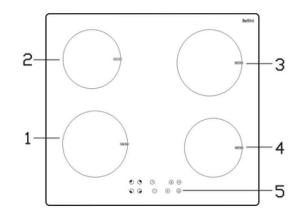
Zone1.max. 1800W/2100 W Zone2.max. 1200W/1500 W Zone3.max. 1800W/2100 W Zone4.max. 1200W/1500 W Rated Input Power :6000W 5. Control panel
