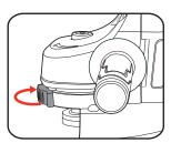
2 Align tabs on the guard with slots on the guard collar and then remove guard.
