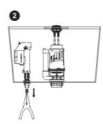
Remove filter from the base of the inlet.
