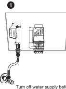
Turn off water supply before cleaning filter. Remove hose connection from the base of the valve.
