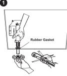
Install valve into the cistern and firmly tighten. Do not use a
