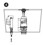
Re-install filter and connect water supply.
