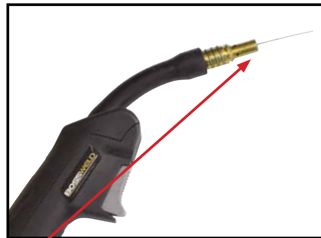
9 Remove nozzle and tip from torch and press trigger on the welding torch, this will feed the wire through the torch. Release button when wire appears at the end of the torch.
