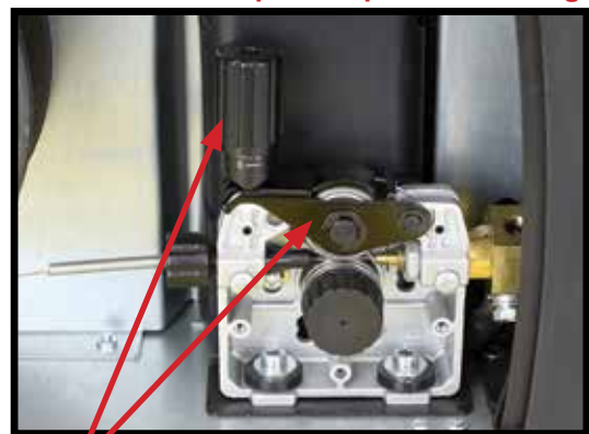
7 Put down Wire Tensioning Arm so it locks into position, and turn the Wire Feed Tensioning Knob to gently tighten.
