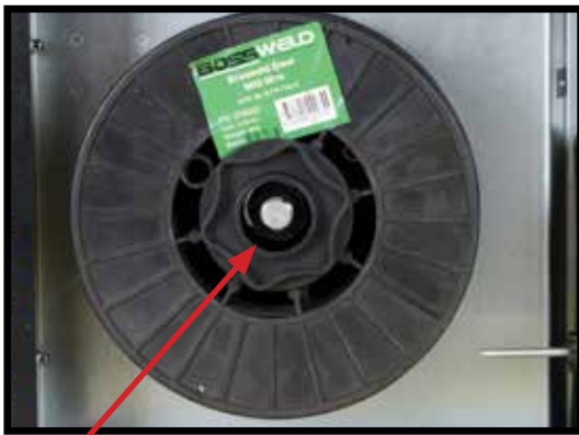
3 Replace Spool Hub Nut and adjust firmly - without too much pressure.
