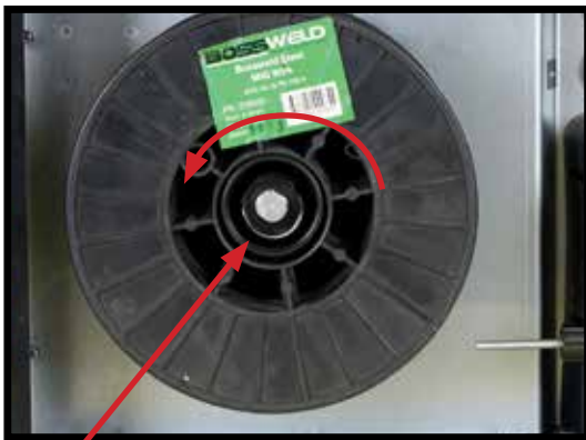
2 Remove the Spool Hub Nut and place spool of wire on Spool Hub. Note: Wire to roll from under spool into wire feeder
