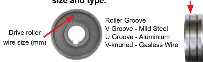
5 Remove the Drive Roller Cover. Check the Drive roller is matched to the wire size for the job Note: Correct wire size side on roller to face into machine when fitting. Then replace the Drive Roller Cover. See Page 16 for drive roller size and type.
