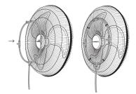
4. Connect the hose connection to the (off) water supply and turn on the fan.
