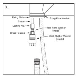
Lock the mixer into position as shown in the diagram above. Ensure the black rubber washer & red fibre washer are installed correctly & a tight seal has been achieved.
