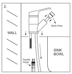
Feed the vege spray hose through the spout, install the hot & cold flexible hoses, install the mixer tap through the sink hole. Ensure the mixer is centred correctly as shown in the diagram above.
