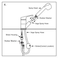
Connect the vege spray hose to the spray head & brass housing using the rubber washers provided. Then install the sinker onto the vege spray hose.
