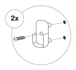
Note – If hanging heavy items, permanently fix the hanger brackets with the supplied screws.
