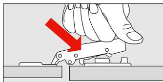
Once hinge is in place, push back of hinge down towards the hinge-plate. Hinge will snap down and engage.
