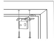
Attach the brackets using the screws provided and a Phillips head screwdriver. Make sure the brackets are firmly in place. For installation in plaster walls use wall plugs provided in the package. Make sure to push the plugs all they way into the wall. Screw the brackets into place, ensuring the leaver of the bracket is facing the front of the blind. Repeat for all brackets supplied.
