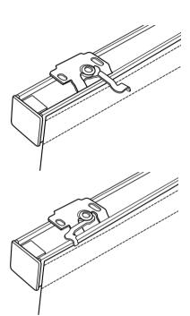
Make sure that all bracket leavers are in the open (front) position before installing the blind.
