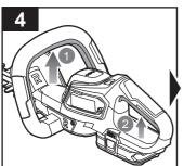
Squeeze the front trigger and the rear on/off trigger simultaneously to turn on the product.
