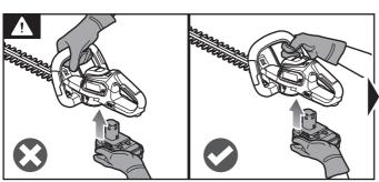
WARNING: Do not hold the top of the front handle when installing the battery pack to avoid starting the product accidentally. Hold the side of the front handle only.
