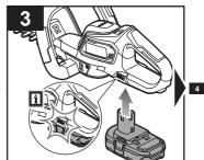
Install the battery pack. Make sure that the latches on the battery pack click into place.
