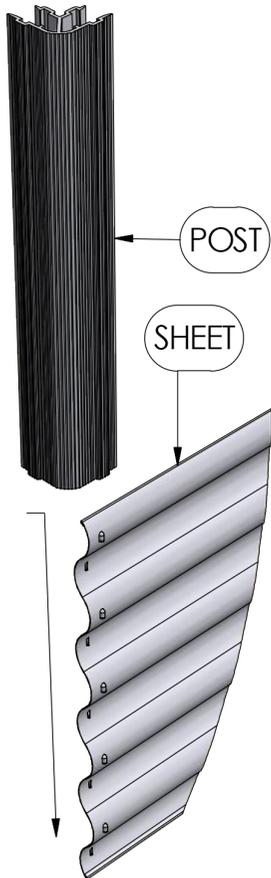
Repeat this for all 4x posts & sheets by; A) installing posts on both ends of 2x sheets, and then sliding the remaining sheets in between those 2x assemblies, or B) working your way around the assembly clockwise or anticlockwise
