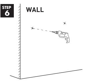
Please perforate holes on the wall based on actual distance between holes for wall mounting.
