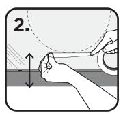
Mark height (x) on door / panel with tape or similar. Cut required hole out above. Hole sizes below 1158 Small: 250mm (9.8") 1159 Medium: 388mm (15.2")
