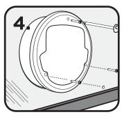
Ensure door is level and secure using the screws provided. Cover screws with screw covers.
