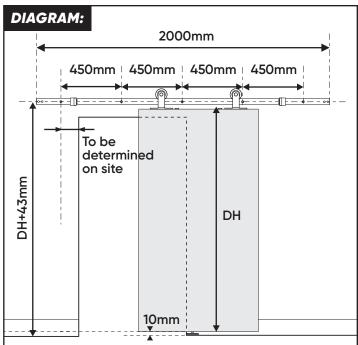
Note: The door size should be a suitable height & width to cover the opening.
