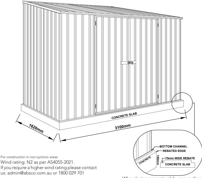
NOTE: This shed can be upgraded to wind rating: C1 as per AS4055-2021 with the additional purchase of a Cyclone Kit.
