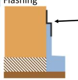
Care must be used when handling flashing to ensure correct fit. Avoid twisting/bending. Flashing is pre-fitted in factory, however it may require gentle manipulation to achieve proper fit.
