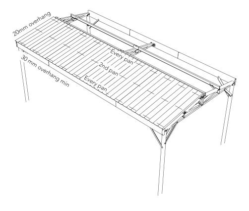
**Option.** On the ground, lay out the roof sheeting as if they were on the frame already. Using a piece of wood, as pictured, turn up the pans of each sheet at the end that's going to be at the ridge.
