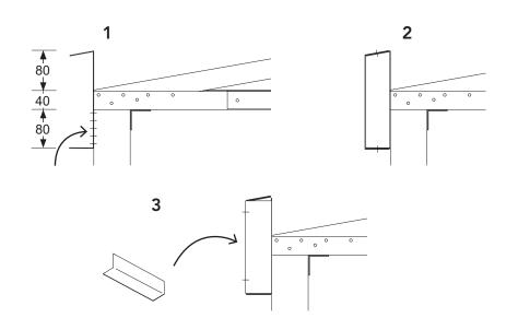
**1.** Safely lift and align the edge beam as shown. It has to sit 80 mm below the post as shown.
