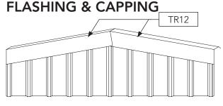
Fit barge capping TR12 to the front and rear gables, fixing where there is a purlin beneath it using tek screws with neo washers.
