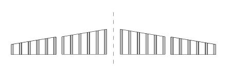
**1.** Take a **050** sheet and using a straight edge, mark the angled line and carefully cut using tin snips.
