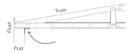
Safely lift a truss and place on top of a pair of posts.
