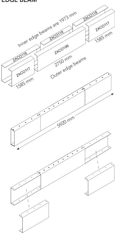
**1.** Arrange the six edge beam pieces as shown on the left.
