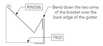
**1.** Attach end caps and join lengths of gutter TR22, to match the length of the edge beam by notching the roller edge of one to allow the other to slide into it.
