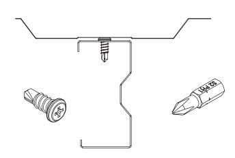
Some holes are pre-punched in Absco sheds' frame sections, however the wide range of positions that most fasteners are required for means that the remainder have to be drilled as per the connection being made
