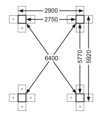
**1.** Place the posts on the foundation, use the dimensions shown to confirm correct placement.
