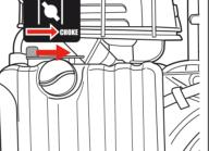
Note: No choke is required If restarting a warm engine, move choke lever to the left position.
