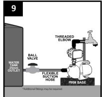
A tap (not supplied) may be equipped onto the end of pipe (not supplied) and secured to the ground with a metal or wooden stake for stability.
