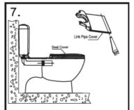
Measure and mark the area to be cut from the link pipe cover by loosely installing the toilet seat into the pan. Remove both items and make the cut with a fine tooth hand saw/hacksaw. Note – Use the cut lines on the back of the link pipe cover to ensure you achieve a straight cut. Reinstall the link pipe cover.
