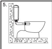
Securely connect the WC pan with the elbow pipe.
