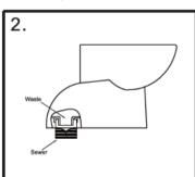
Connect the waste to the sewer, ensure that the sewer connection is connected correctly and that a good seal has been achieved.
