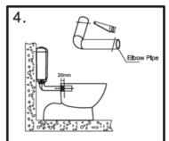
Cut the elbow pipe to size before connecting it to the WC pan connector. Note – Use a fine tooth hand saw/hacksaw to make the cut, ensure there is a 20mm minimum connection into the pan.
