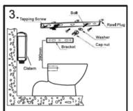
Hang the bracket on the wall. Note – Take caution when selecting the area to be drilled as water pipes or other hazardous objects may be present in wall. Install the cistern.
