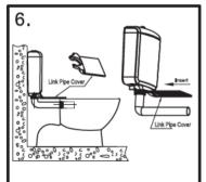
Install the link pipe cover on the cistern.
