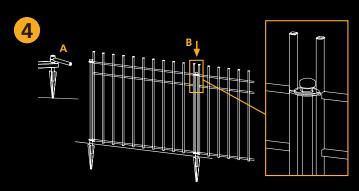
A: Hammer the second spike into the ground at the marked location.
