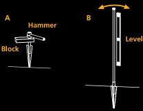
A: Position the first spike and hammer it into the ground until the top of the blades are flush with the surface.
