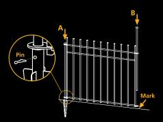
A: Insert the first post through the fence panel tabs and down into the spike. Then secure with pin (provided).
