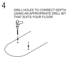
DRILL HOLES USING AN APPROPRIATE DRILL BIT. APPLY WET AREAS SILICONE INTO THE HOLES & TO THE BASE OF THE FLOOR BRACKET TO HELP KEEP THE FLOOR WATERPROOF, INSTALL THE FLOOR BRACKETS INTO POSITION. DON'T INSTALL SS SCREWS AT THIS POINT.
