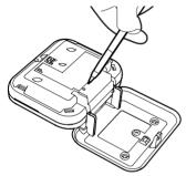
Using a ballpoint pen, briefly push and release the 'learn button' on the back of Alarm 2. The red LED next to the learn button will flash briefly then light up for approximately five seconds.
