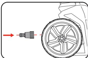
**Note:** The hose adaptor is fitted with a mesh inlet filter. This filter must be in place to prevent impurities in the water source from entering the unit and damaging the pump.
