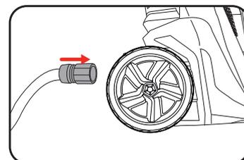
**Note:** A filter is fitted to the hose adaptor preventing any debris from entering the pump. Inspect and clean the filter before use as insufficient water supply could damage the pump.
