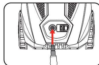
2. Gently tug on the high pressure hose to check that the connection is secure.
