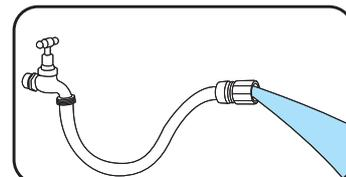
2. Attach garden hose (min.Ø 1/2") to the hose adaptor on the water inlet port of the unit. Always use a reinforced hose with a standard coupling for water inlet. The hose length **can not be greater than 8m in length** for proper operation.
