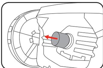
2. Screw supplied hose adaptor onto water inlet port.
