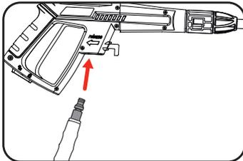
4. Gently tug on the high pressure hose to check that the connection is secure.
