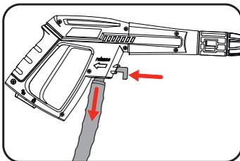
**Note:** To disconnect the high pressure hose, press and hold the quick-release and pull out the high pressure hose.
