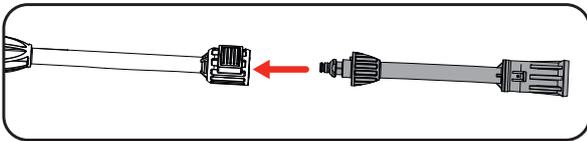
**Note:** To disconnect the adjustable spray nozzle, press and hold the quick-release on the extension lance and pull out the adjustable spray nozzle.
