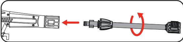
2. Push the adjustable spray nozzle into the connector end of the extension lance until it clicks into place
