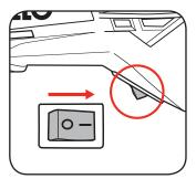
2 To turn off, push the on/off switch to the off position "0".
