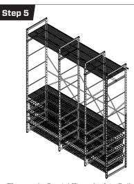
Please note: For stability and safety, fix the unit to a wall with the provided brackets. Place the brackets over the rear frame legs at the top and bottom, then attach to your wall. Necessary fixings for these brackets can be found at your local hardware store.
