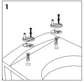
Install washers (F) onto screws. Insert components (B), (C), (E) and (D) into the pan.
