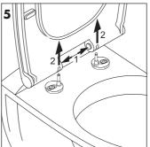
Remove seat **6** by pressing the release buttons, then lifting it upwards.
