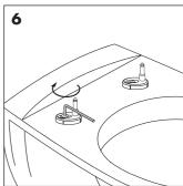
Fully tighten the screws © in a clockwise direction.
