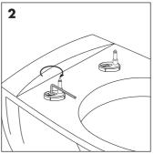
Semi-tighten the screws © in a clockwise direction. Do not fully tighten, as the position of the hinges ® may need to be adjusted.
