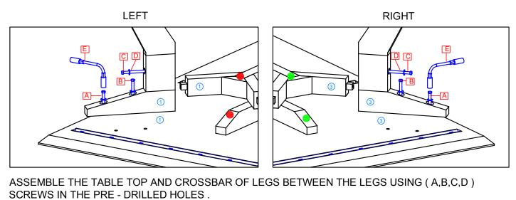
TIGHTEN WITH ALLEN KEY ( E ) ONCE ALL SCREWS HAVEN BEEN SECURED IN PRE - DRILLED HOLES .
