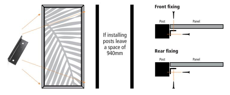
**2.** Use ProtectorAl Decorative Screen In-ground (2400mm) Post with multi-angle post slots for easy fitting Important: Screens should be positioned a minimum of 600mm from all heat emitting sources in a ventilated area.
