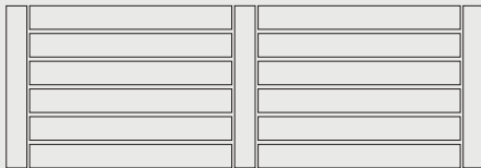
Example of a breaker board design (recommended for decks longer than 5.4m):
