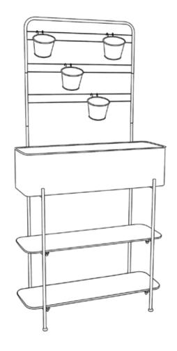
NOTE: To avoid possible twisting of frame, do not tighten screws completely until fully assembled.
