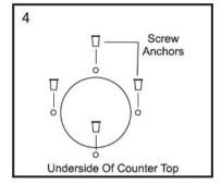
Insert each screw anchor into each drilled hole.
