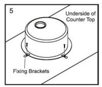
Place the fixing brackets over the screw anchor's and loosely tighten into position. Using the screws provided. Align sink into desired location.
