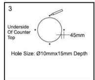
Drill into the underside of the counter top as shown in the diagram above.
