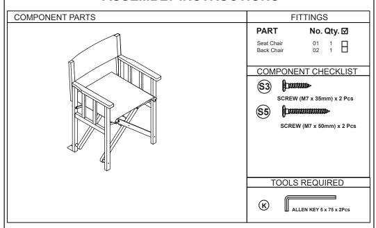
Step 1 Partially open the chair then attach the back rest timber uprights to the chair at the pre-drilled holes using screws S3x2 and S5x2.
