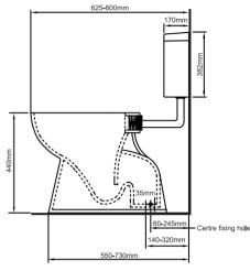
IMPORTANT NOTE: These dimensions are provided solely as approximations only. It is crucial to verify all measurements with your specific toilet before starting the installation, particularly before any drilling into walls for bracket placement. If you are installing your toilet on a cement bed, please take this into consideration.
