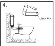
Cut the elbow pipe to size before connecting it to the WC pan connector. Note – Use a fine tooth hand saw/hacksaw to make the cut, ensure there is a 20mm minimum connection into the pan.
